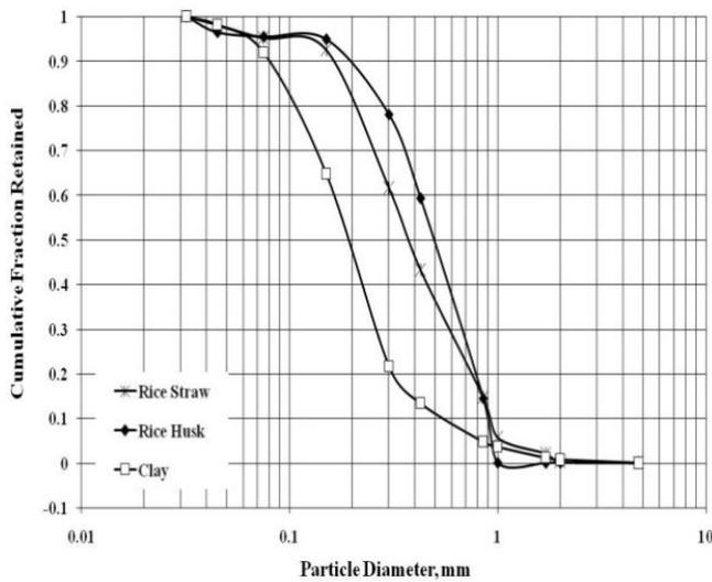
**Figure 1: Cumulative Screen Analysis of Raw Materials**
