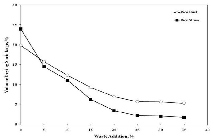
Figure 12: Effect of Waste Addition on Volume Drying Shrinkage
