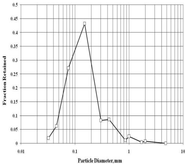
**Figure 2: Differential Screen Analysis of Clay**
