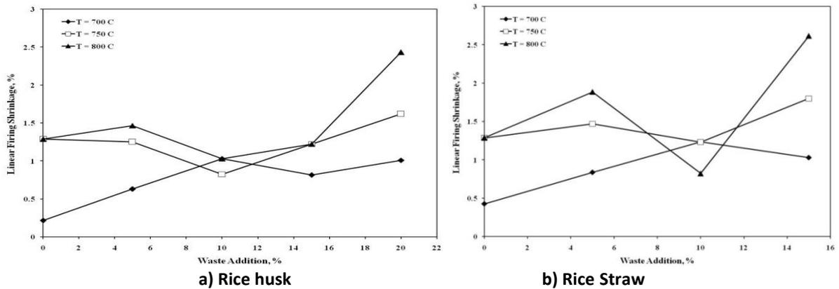
Figure (14) Effect of Waste Addition on Linear Firing Shrinkage
