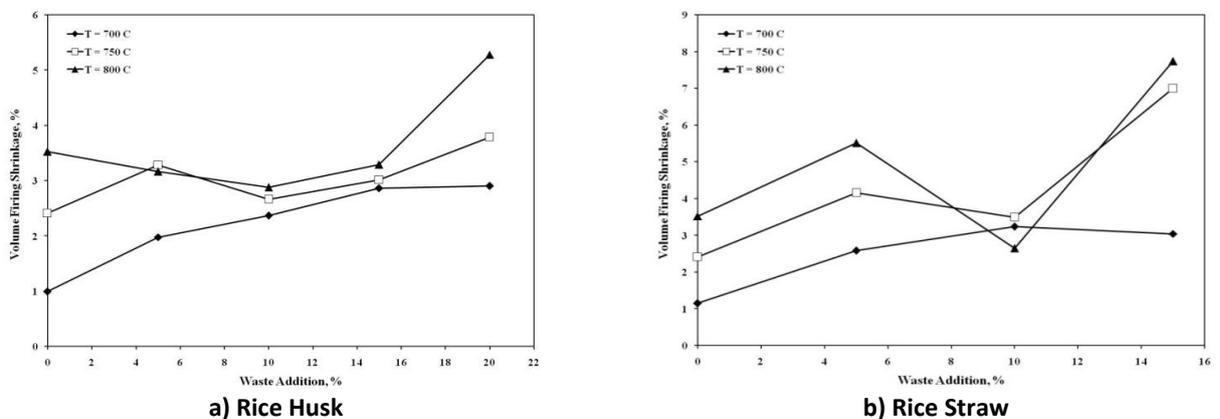
Figure 15: Effect of Waste Addition on Volume Firing Shrinkage,
