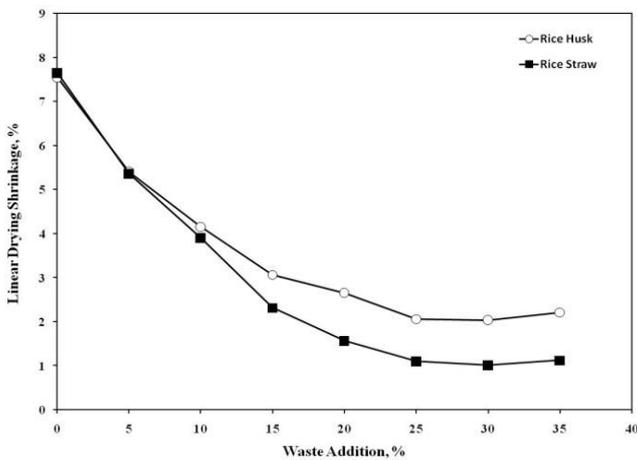
Figure 11: Effect of Waste Addition on Linear Drying Shrinkage
