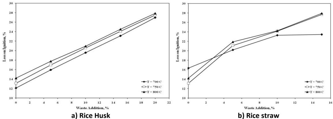
Figure 13: Effect of Waste Addition on Loss Ignition of Fired Samples
