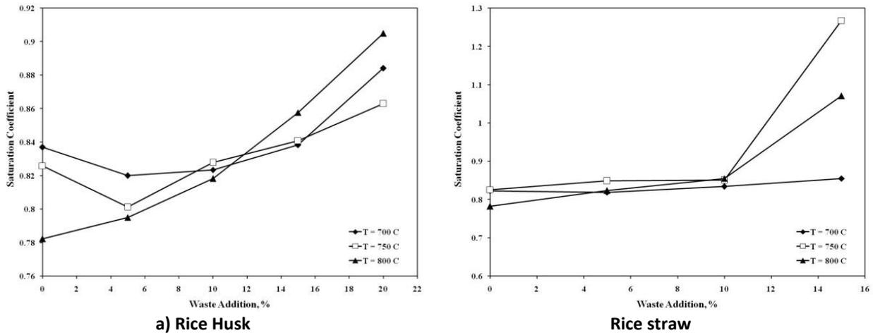
Figure 18: Effect of Waste Addition on Saturation Coefficient, a) Rice Husk, and b) Rice Straw
